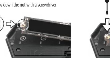
B Screw down the nut with a screwdriver
