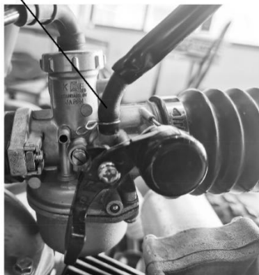
Tank fuel pipe docking completed
