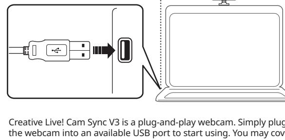
Creative Live! Cam Sync V3 is a plug-and-play webcam. Simply plug the webcam into an available USB port to start using. You may cover the lens with the attached Privacy Lens Cap when the webcam is not in use to ensure privacy.
