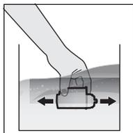
Hold the water filter cartridge under cold water and gently agitate it to remove all the air bubbles.
