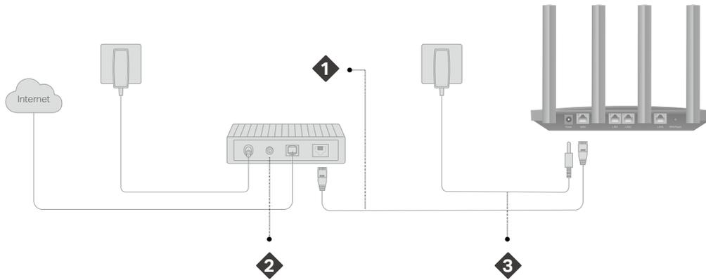
1. Connect the modem to the router's WAN port with an Ethernet cable.
